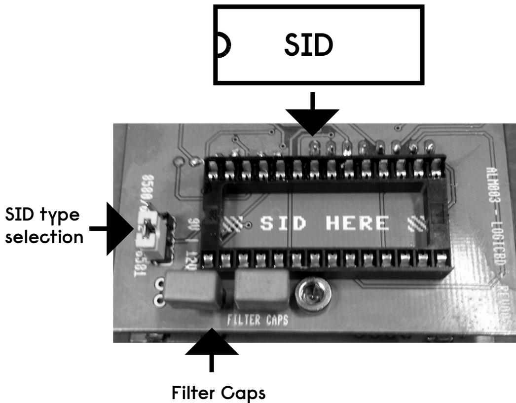
The SID GUTS supports 3 different types of SID chip; The original 6581 chip, the later 8580 and a modern hardware emulation chip - the 'SwinSID'. The SID chip should be clearly identified. Beware of fake SID chips or partly working SID chips with broken filters.
