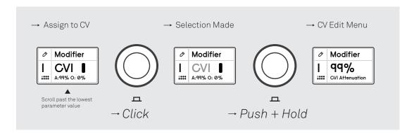
The set attenuation value can be either positive or negative which in effect inverts the CV value (i.e just like an attenuverter)
