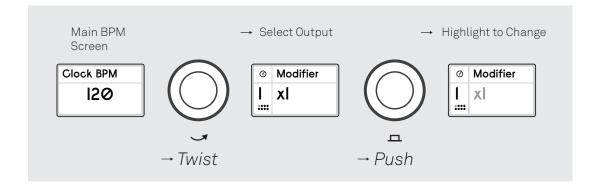
Each output is represented by the output number (on left) together with the current set modifier value for that output. The modifier value is either a multiplier, a divider or a 'utility' value correlated to the set BPM clock speed.
