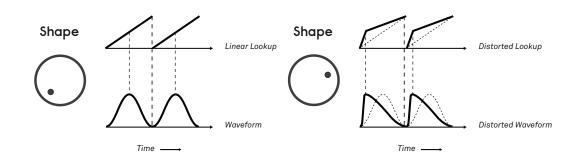
The shape is set by the offset and associated CV input, with an attenuverter to attenuate and invert the CV.
