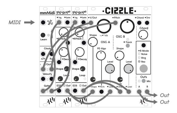
Tip: The two voices can be independently patched for further processing or mixed together in stereo by engaging the Mix switch.
