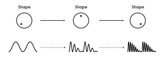
The shape is set by the offset and associated CV input, with an attenuverter to attenuate and invert the CV.
