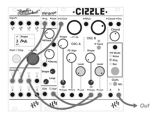
Tip: For wider ranging more experimental ring mod sounds disengage the OSC B track switch, unlocking the two oscillator frequencies and allowing them to be set freely.
