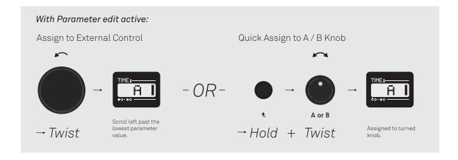
Any number of parameters can be assigned to the same source for macro control. Furthermore, each assignment includes its own digital attenuation and offset settings for scaling the incoming modulation. To adjust this, hold the program encoder for >1 sec. with the assignment selected. (To exit press the back button). When a source is assigned, a small bar graph will be displayed indicating the modulation level (after attenuation and offset).
