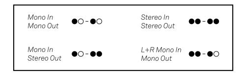
All reverbs (except the Pocket PL8 & Slinky Reverb) preserve the stereo dry input signals when performing the mix with the wet signal.
